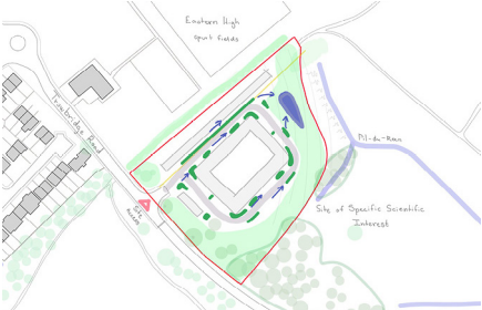
04 SUSTAINABLE DRAINAGE INTEGRATED INTO PLACEMAKING THE DRAINAGE STRATEGY WILL INCORPORATE SITE-WIDE RAIN GARDENS, SWALES AND A FEATURE ATTENUATION POND. THEY ARE EMBEDDED WITHIN THE SCHEME AND ARE USED TO HELP DEFINE THE CHARACTER OF THE DEVELOPMENT.
